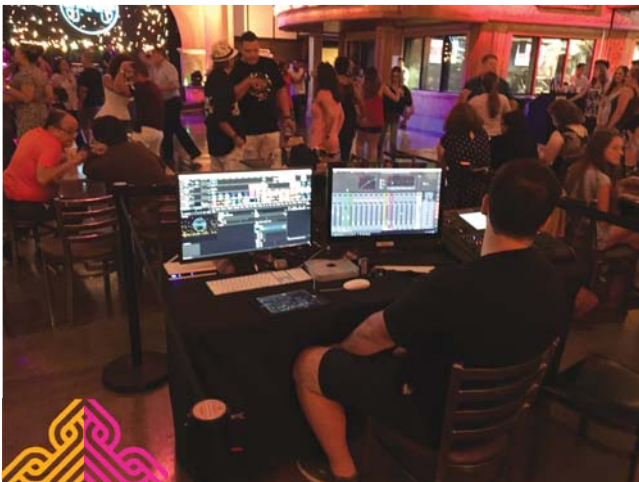
Plaza Mariachi's front-of-house position is on the dancefloor, with conduit cabling to the PA and lighting, and with iPad control that allows the mixer to listen in various areas of the room.
